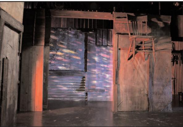
The arresting effect in the window of this set was created with Rosco's standard steel Dots Breakup (Medium) gobo 77053 in one slot of the rotator and the Sunset Prismatic (glass) gobo 43804 in the other slot.
